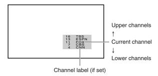
Repeatedly press or hold Channel ▲ or ▼ while the SpeedSurf mode is on-screen to scroll the channel list. Release the button to display the highlighted channel.
